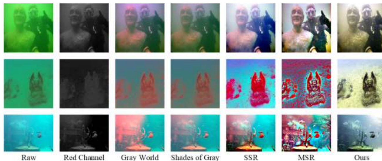
Fig. Underwater color correction results. Applying color correction directly will produce severe red artifacts.
